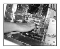
**Step 5**Locate an available PCI expansion slot. This will be in the area of your computer where other cards that look similar to the PYRO PCI card are installed.
